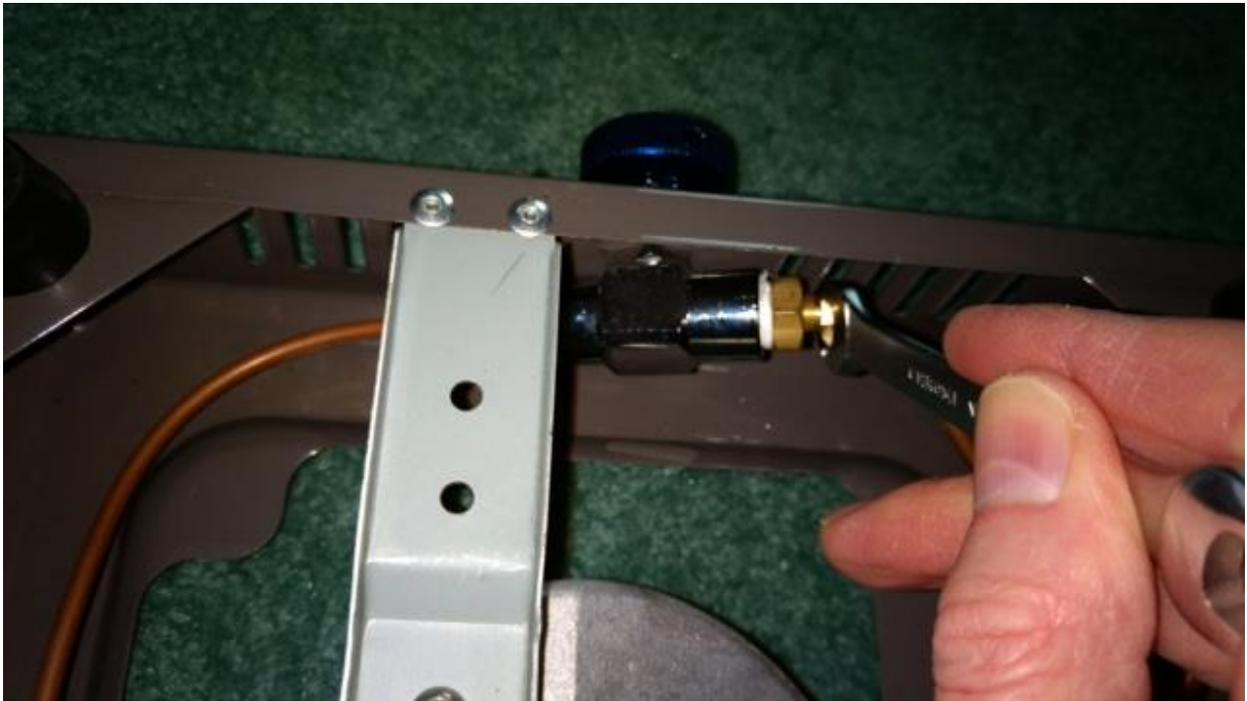
3. Remove the nut that fastens the body of the valve to the burner housing. This will allow you to remove the valve.
