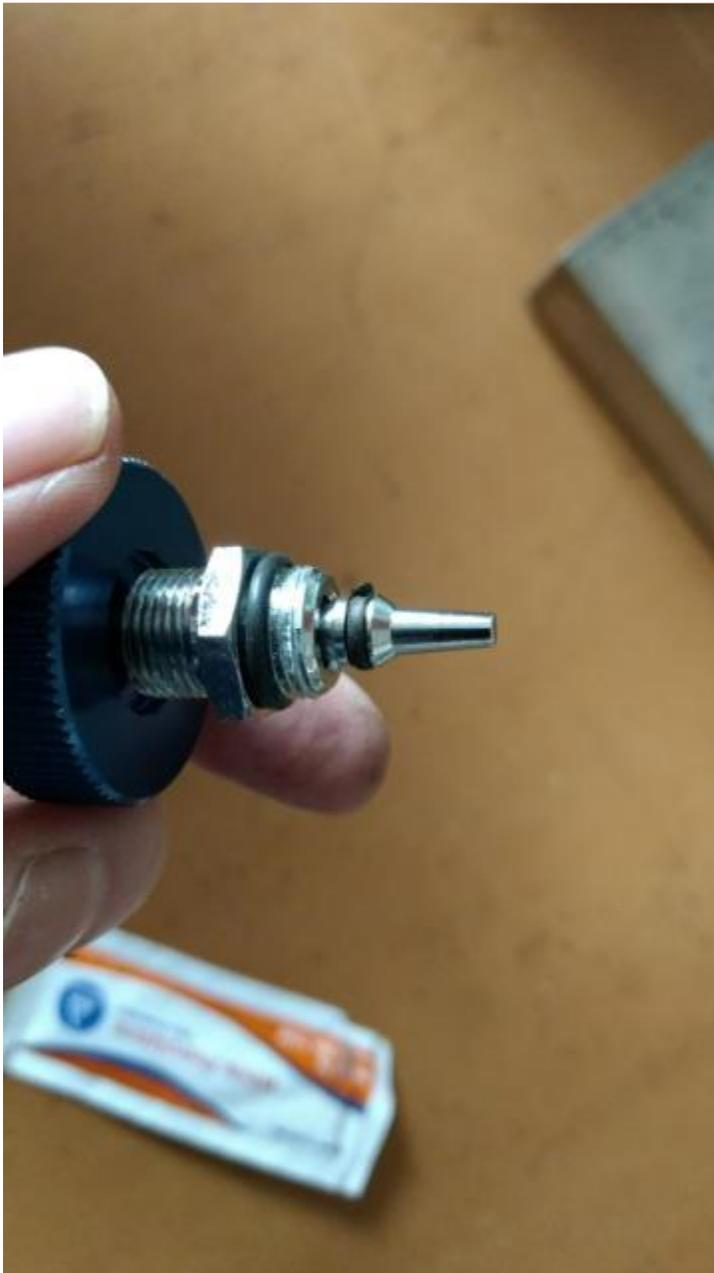
1. To remove the valve first remove blue knob and locking nut from the needle valve stem. You will need a hex key to loosen the set screw in the knob.
