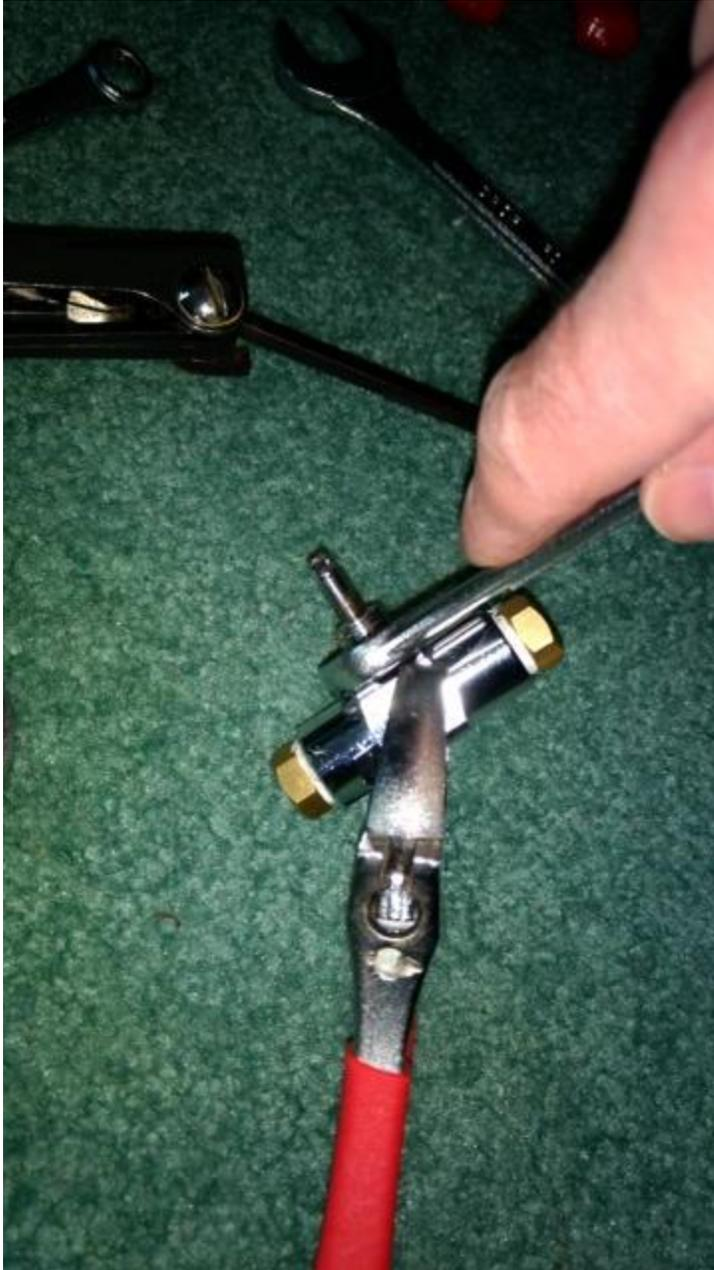
5. Thoroughly clean the moving parts of the assembly by screwing the stem in as far as it will go. This exposes the stem and needle with the O-ring (see the first photo). After cleaning apply a small amount of Dow 111 to the O-ring.
