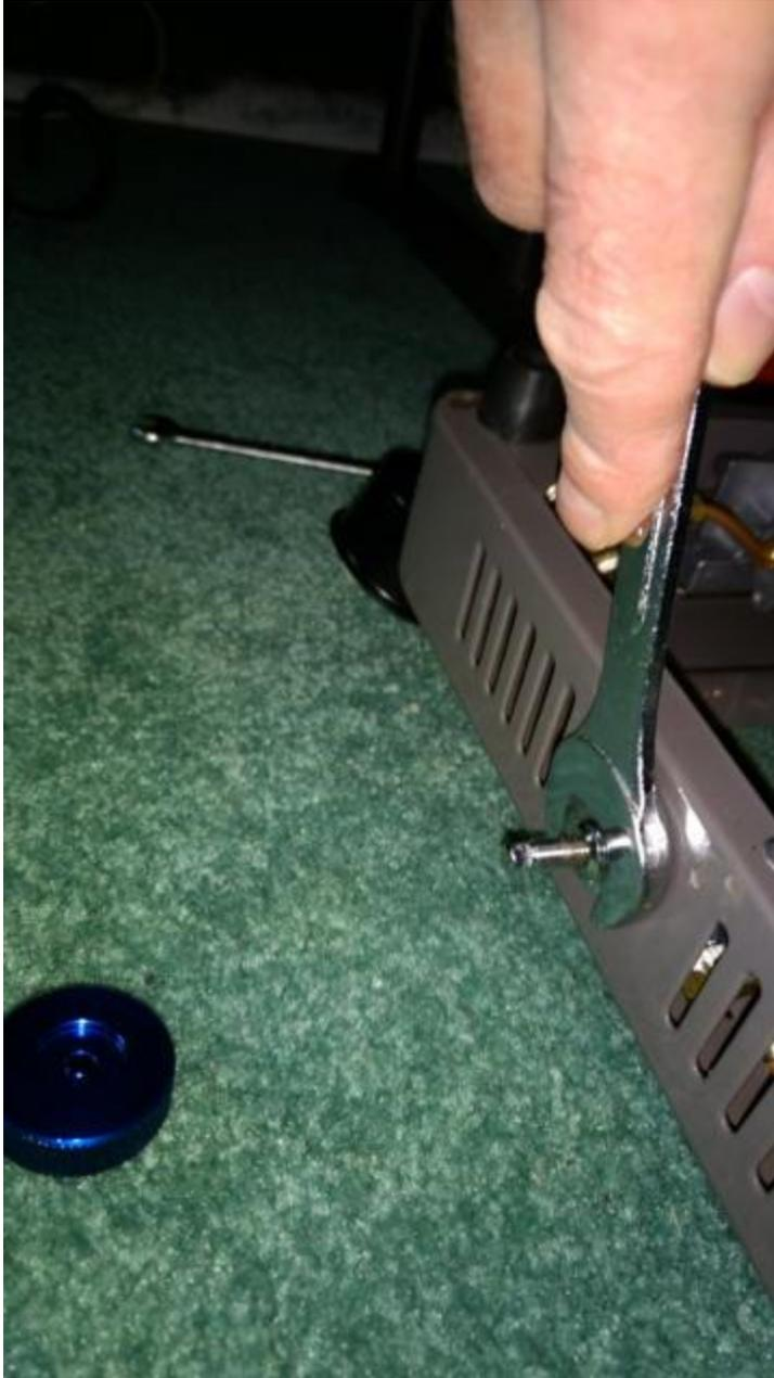
4. Remove the packing nut from the valve. If you have a vice that should make things easier. I was able to put a box end wrench on the packing nut and an adjustable wrench on the square section of the valve body. The packing nut had joint compound on the threads. I didn't have any but used Teflon tape when I screwed it back in. If you use Teflon tape you must be very careful not to allow any excess tape to drape around the end of the threads which could block the opening.
