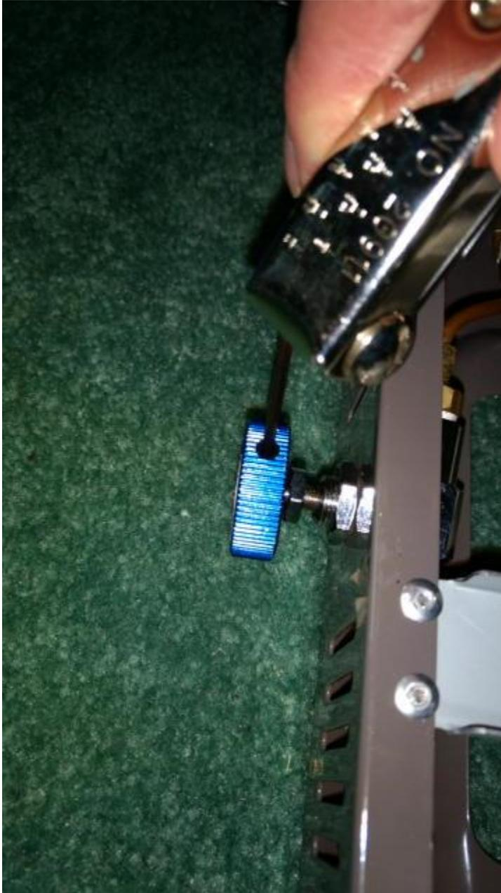
2. Remove the two 1/8" compression fittings from the valve inlet and outlet. It's best to remove the longer copper tubing first. The longer tubing gives the pipe more flexibility which facilitates removing the nut. Once the nut has been backed off far enough to remove the tube from the valve, there will be nothing to impede the removal of the shorter 1/8" tubing.
