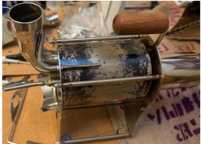
Once you've successfully taken out all the screws, the shroud should slip off with ease and leave you with a Huky in the nude. (In the picture to the right you can see how the MET is attached to the frontplate. If you didn't order a MET thermocouple, there's a nut and bolt instead. The BT is attached in the same way.)
