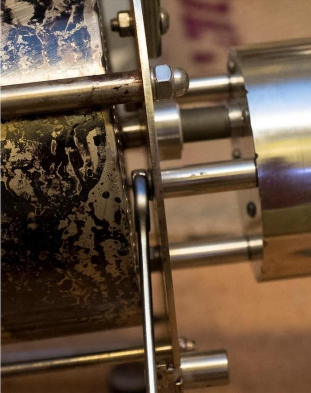
First, you should put the motor assembly in place before setting the drum in place. To make sure that these two align, don't tighten the nuts before you've felt that the drum is spinning freely with the motor. Once you've attached the front plate, you can tighten the nuts for the motor after a test run. If there's some kind of noise, it's easy to wiggle the motor a bit to find the "silent spot" and then tighten the nuts.
