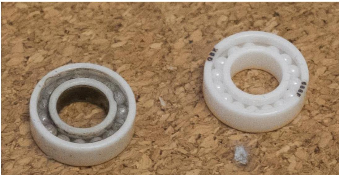
Important: There's an orientation of the bearings, which is just about seen on the picture above (on the left bearing). There's a slight indentation at 10 o'clock in the outer ring and at 2.30 in the inner ring. These indentations must face inwards in the bearing holders. I.e. put that side inwards, towards the drum on both sides.
