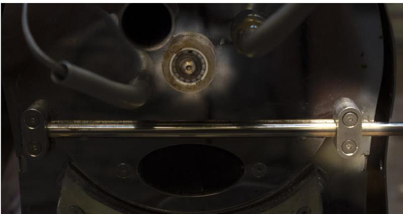
It's enough to unscrew the two highlighted screws in the picture above. Then you can pull out the hatch and put it aside (after cleaning ☺).
