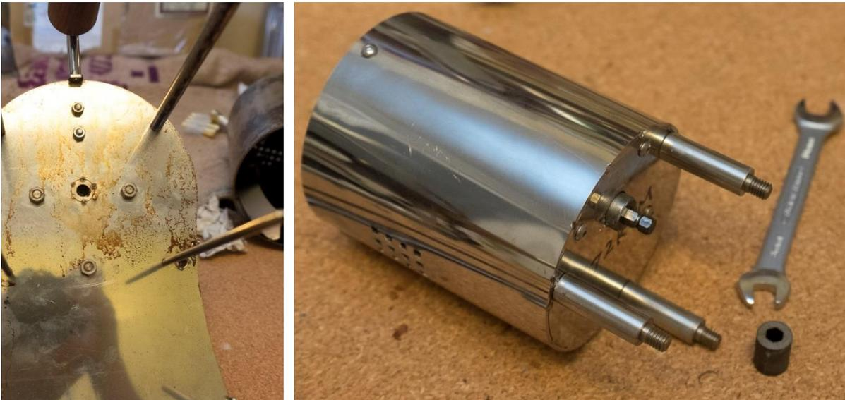
The motor is held in place with 3 10mm nuts (don't lose those washers...). I think that the small black coupling between the motor and the drum still is the current model, but I know that there are older versions where which that coupling was more prone to getting lost.
